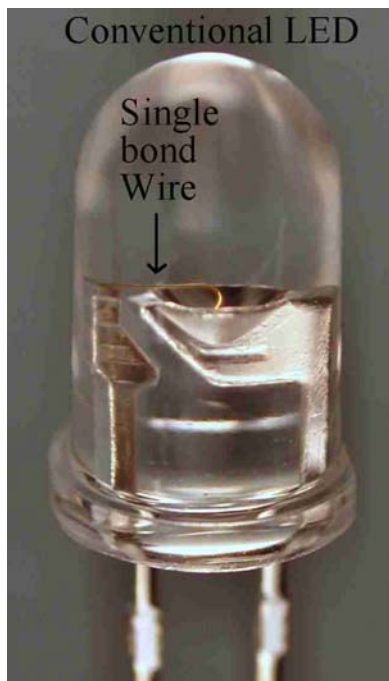
Fig. 4 — Conventional LED wire bonding, single bond wire.
