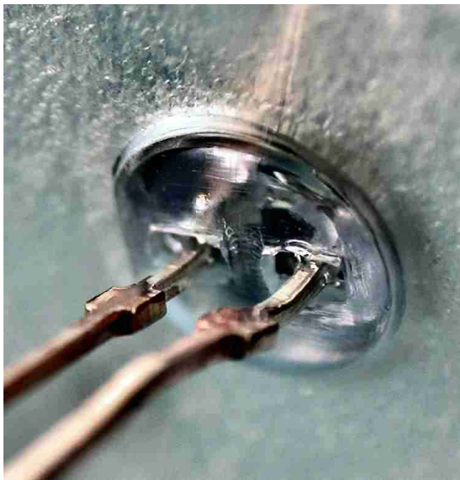
Fig. 11 — Flat rigid LED leads pass through the LED chamber wall and are soldered onto the circuit board. See figure 12 for a circuit board chamber overview.
