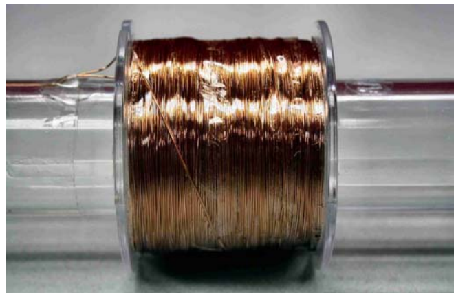
Fig. 23 — FFL coil form width wound with 30 Ga. wire.
