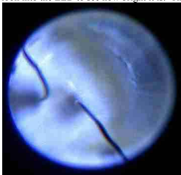
Fig. 3 — The lens magnifies the two 1 mil diameter LED bond wires to make them more visible.
